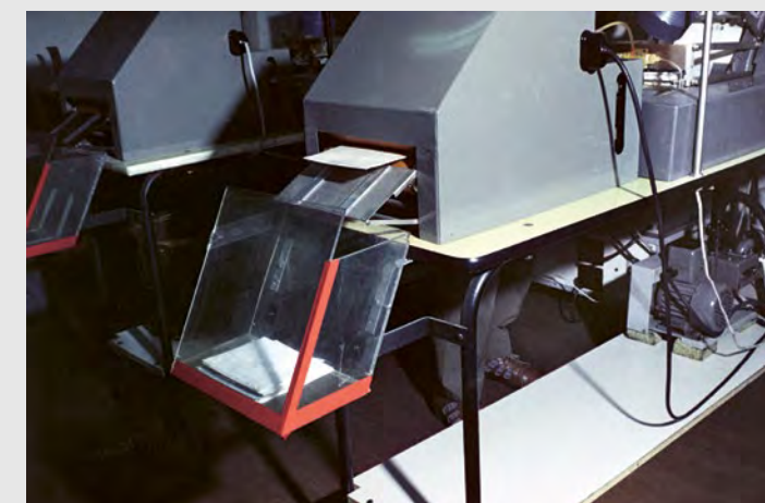
58 → Checked letters are reclosed in a letter sealing machine, around 1984.
